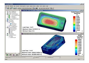
ALGOR FEMPRO's Superview IV Results environment enables engineers to view different types of results in multiple view windows. In the lower frame, the viewport is displayed transparently to reveal the stresses inside the housing.
