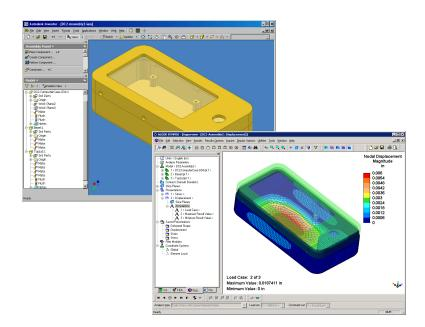
ALGOR's InCAD technology provided direct CAD/CAE data exchange of this oceanographic instrumentation housing from Autodesk Inventor (top) for a linear static stress analysis (bottom).
